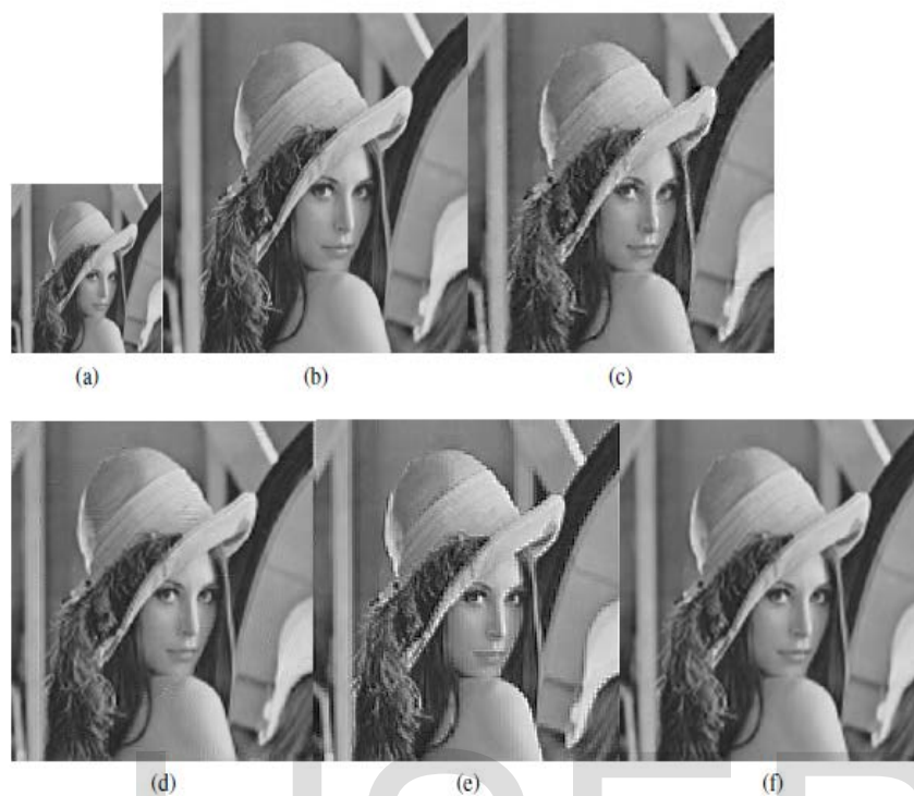
Figure 3: (a)Low resolution image (b)Original image (c)Freeman method(d)wavelet method 1(e) Sapan's wavelet method[21] (f)block wavelet method
